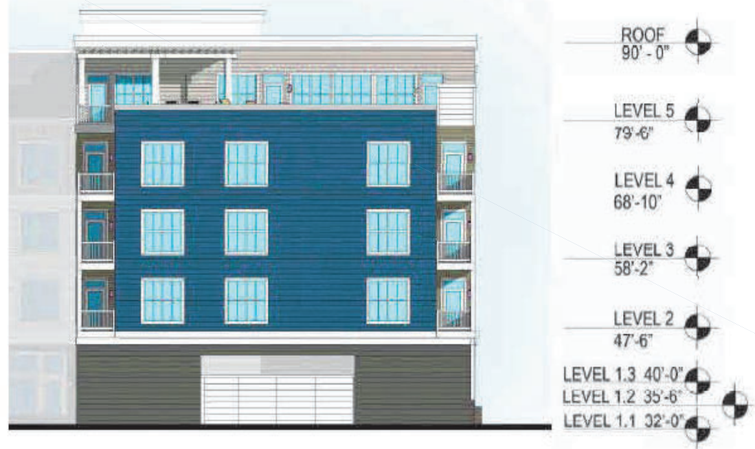
13 EXTERIOR ELEVATION SOUTH WEST - PITMAN ROAD Scale: 1/16" = 1'-0"
