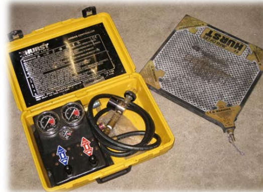
Current set of air bags purchased in 2004 and are past recommended life span
