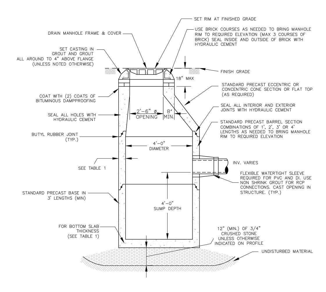
DRAIN MANHOLE DETAIL (TYP.)
