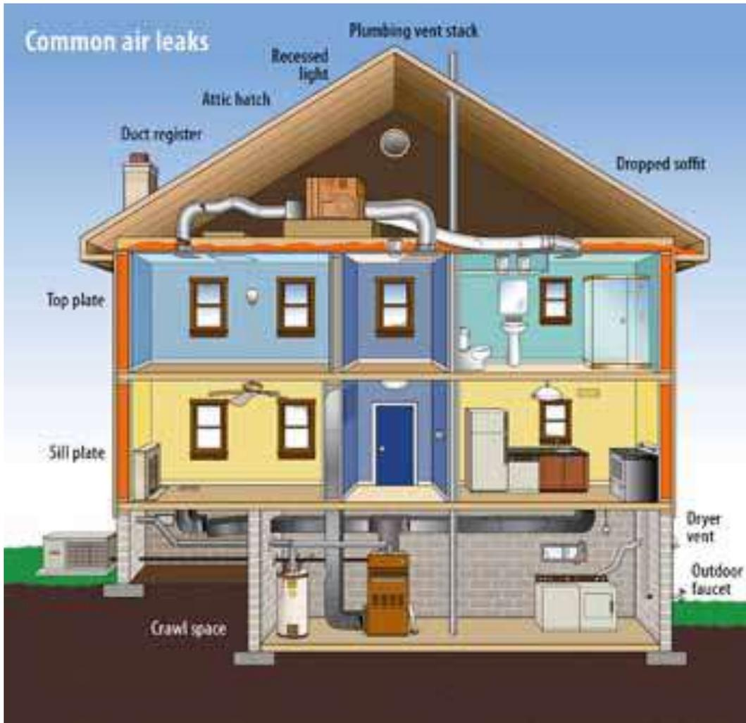
Prescriptive codes don't guarantee good installation, air and water tightness, or that thermal insulation is effective. (small air gaps can reduce insulation R-values by 50% or more)
