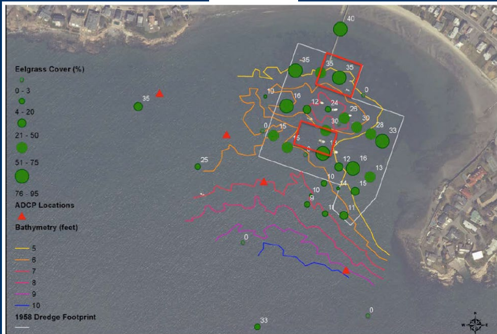
Figure 7. Alternative #4, the Reduced Impact Plan, showing the boat mooring area outlined in red, inside the 1958 Dredge Area. Alternative #4 reduces the impact to eelgrass by dredging smaller areas in the shallowest parts of the mooring area.
